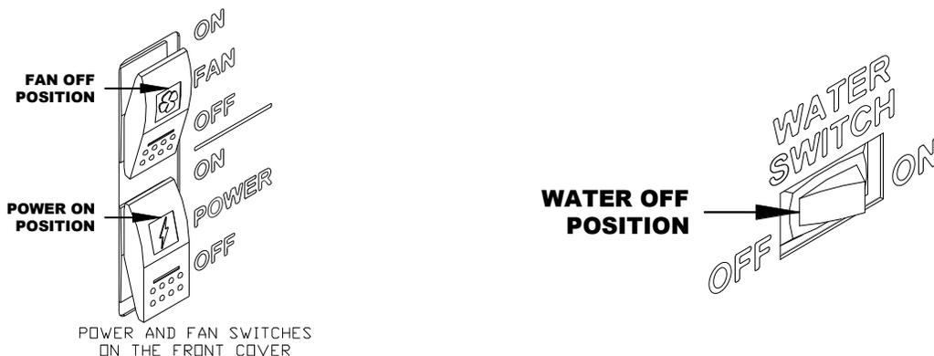
**Steam Sterilization Operation Switches Diagram**
